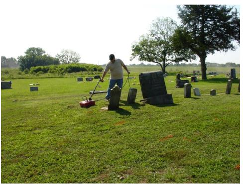
Ground penetrating radar was employed to determine where burials were and which plots were empty.
